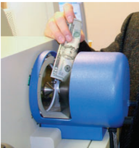
DART ionizes molecules on the surface of a $20 bill.
