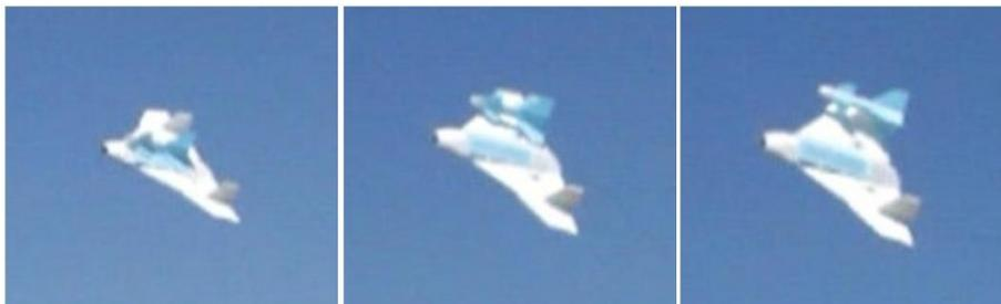
*Figure 9. Drop vehicle catching on vertical tail.*
