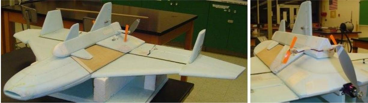
Figure 2. Primary UAV, Drop Vehicle and Interior Search Vehicle
