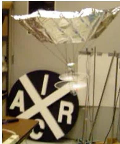
*Figure 7. Hover test with faceted stabilizer.*
