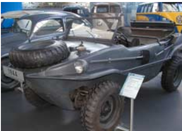
This is a WWII amphibious jeep known as a Schwimmwagen. There was also a Kublwagon (what the VW Thing was modeled after)... WWII jeep, and WWII
