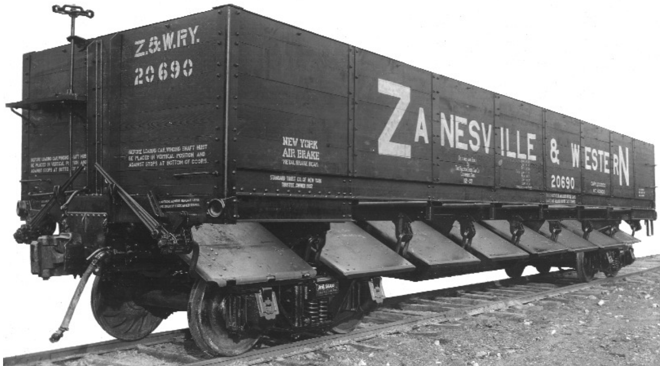
FIGURE 4.8 Zanesville & Western car number 20690 was built by the Ralston Steel Car Company in December 1907. The car had an inside length of 40' 0", inside width of 9' 3", inside height of 4' 6 1/4", and height to top of sides of 9' 0". It had a capacity of 1,665 cubic feet and was rated for a load of 100,000 pounds. The self-clearing, side-discharge design was based upon a 1904 patent by Anton Becker, who partnered with Joseph Ralston to form the company in Columbus, Ohio. This design was popular with a number of railroads. Note the instructions for the door operating mechanism posted at the end of the car. [ Ralston Steel Car Company Photo; Courtesy: Alexander J. Campbell Collection ]
