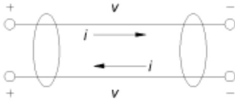
Figure 1 - Transmission Line in Transverse (TEM) Mode
