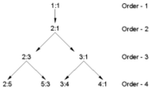
Figure 4 - Voltage Transformation Ratios of the First Four Orders of TLTs (from Rotholz [6])
