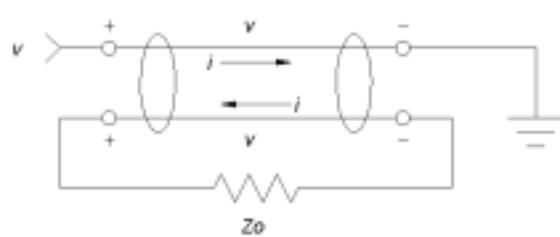
Figure 7 - Order-1 Transmission Line Transformer Used as a 1:1 Current Balun
