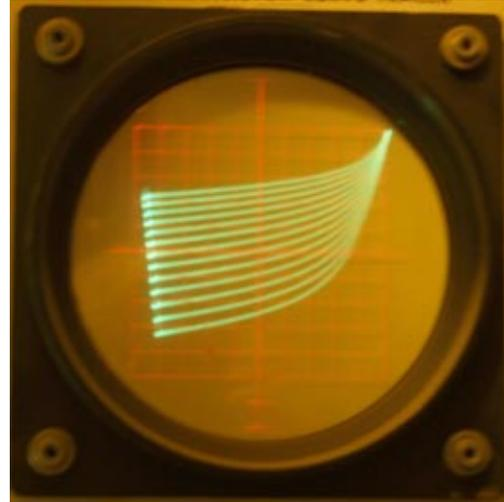
Fig. 2F - 2N5462 (100mV/step, vertical - 0.5mA/div, horizontal - 1V/div)
