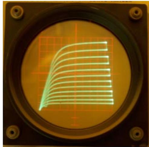
Fig. 1K - 2N5486 (200mV/step, vertical - 1mA/div, horizontal - 1V/div)
