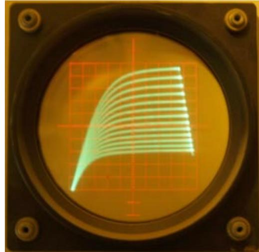
Fig. 1E - J310 (200mV/step, vertical - 5mA/div, horizontal - 1V/div)
