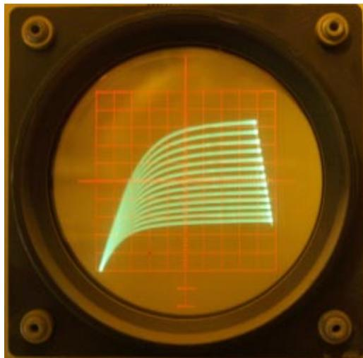
Fig. 1C - BF244C (200mV/step, vertical - 2mA/div, horizontal - 1V/div)
