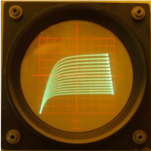
Fig. 1B - BF244B (100mV/step, vertical - 1mA/div, horizontal - 1V/div)
