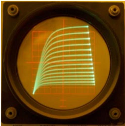
Fig. 1G - MPF102 (200mV/step, vertical - 1mA/div, horizontal - 1V/div)
