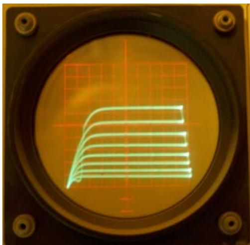
Fig. 1J - 2N4416 (200mV/step, vertical - 1mA/div, horizontal - 1V/div)
