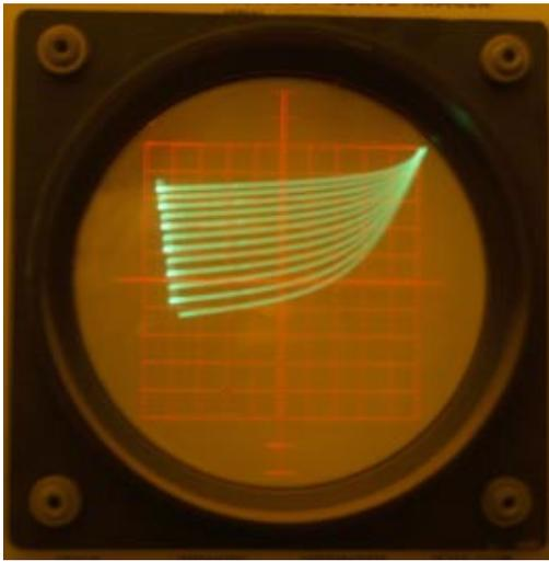
Fig. 2A - J174 (200mV/step, vertical - 5mA/div, horizontal - 1V/div)
