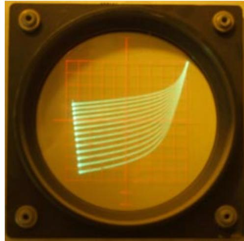
Fig. 2E - 2N5461 (100mV/step, vertical - 0.5mA/div, horizontal - 1V/div)
