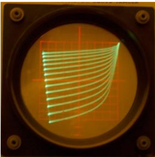
Fig. 2C - J271 (100mV/step, vertical - 1mA/div, horizontal - 1V/div)
