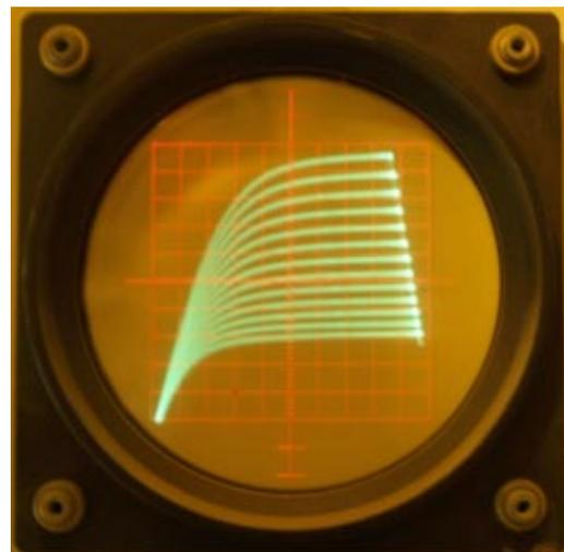
Fig. 1F - U310 (200mV/step, vertical - 5mA/div, horizontal - 1V/div)
