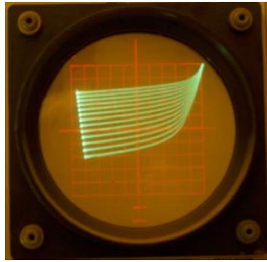
Fig. 2D - 2N5460 (100mV/step, vertical - 0.5mA/div, horizontal - 1V/div)
