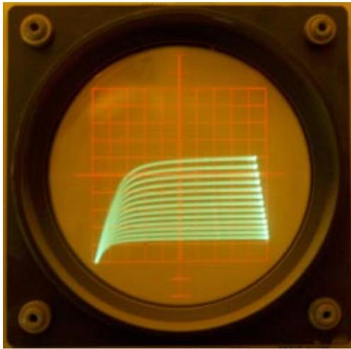
Fig. 1A - BF244A (100mV/step, vertical - 1mA/div, horizontal - 1V/div)
