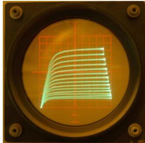
Fig. 1D - J309 (100mV/step, vertical - 2mA/div, horizontal - 1V/div)
