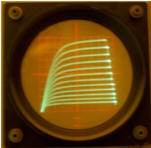
Fig. 1H - 2N3819 (200mV/step, vertical - 1mA/div, horizontal - 1V/div)
