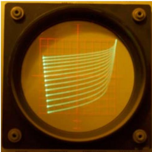
Fig. 2B - J270 (50mV/step, vertical - 0.5mA/div, horizontal - 1V/div)
