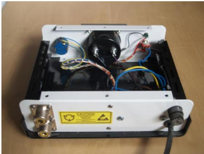
Fig. 9 - Active Antenna Power and Control Unit Prototype
