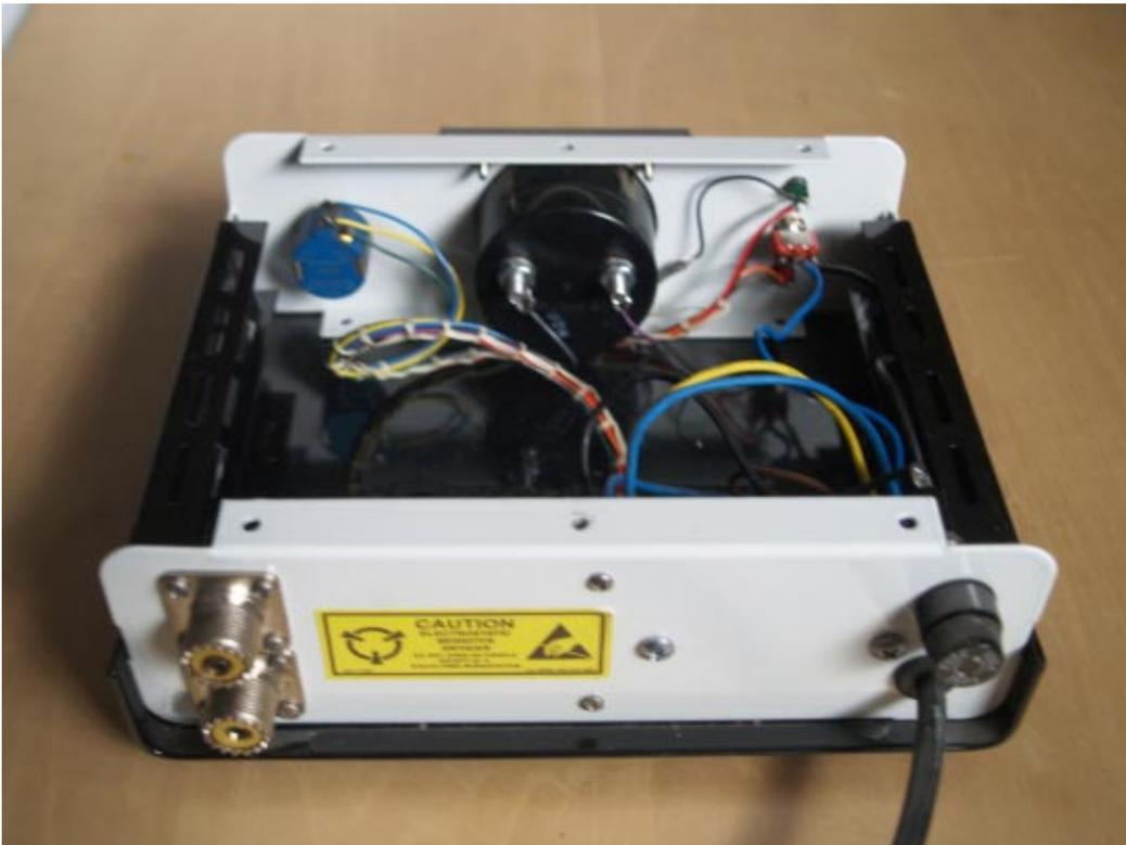
Fig. 14 - Active Antenna Power and Control Unit Prototype
