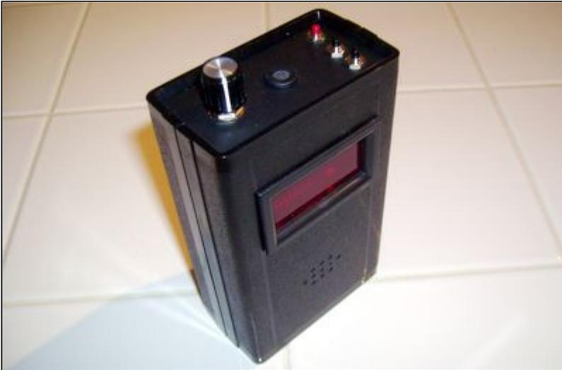
The Bat Scanner is a heterodyne bat detector that has advanced automatic scanning capabilities built into it. The frequency is adjustable in 2kHz increments from 10kHz to 80 kHz.
