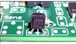
Now install the [LP2950A](#) , a 5 volt regulator IC, on the PCB.
