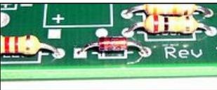
Install the 6 volt, [1N753A](#), glass packaged zener diode ... with the banded end oriented toward the 220 ohm resistor, as shown on the PCB silk-screen.
