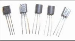
The next step is to sort out the transistors and regulator IC. These look very similar. It helps to note that there are four transistors, and only one regulator IC.
