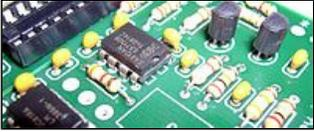
There should be five spots left on the circuit board for the five remaining [.01uF](#) caps. The [.01uF](#) caps are marked [103](#). Once these are in place, the small caps are done.
