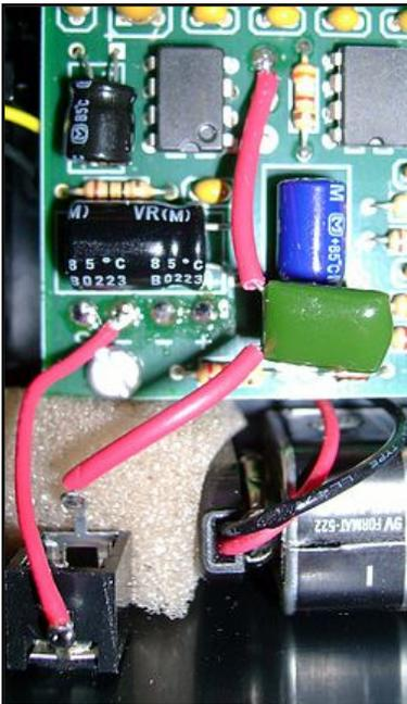
This picture shows a tape recorder output jack installed on the bottom panel. A single circuit, 3.5mm phone jack is mounted in the upper left corner of the bottom panel.
