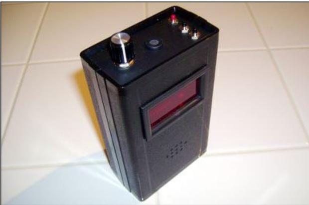
Refer to the [User Guide](#) and follow the procedure for setting the [SENS](#) pot. Once this is done, you can close up the finished detector with the two long self tapping screws. These screws can be hard to screw in and remove when the case is new ... you may want to drill out the bosses just slightly with a 3/32" drill bit ...
