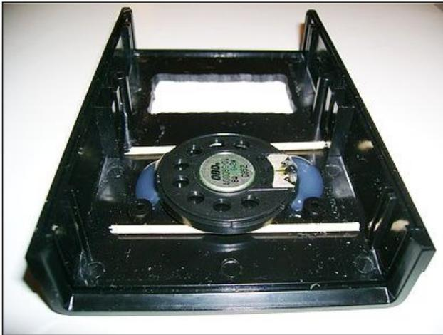
Once the front case has been drilled, and all the rough edges cleaned up, it is time to install the speaker. The method I've adopted sets the speaker back from the front of the case a little bit, which seems to give the detector better overall sound quality.
