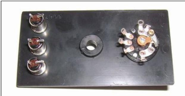
From the back you can see how the soldering connections are aligned. I like to use shielded wire for the microphone to minimize picking up internal noise from the display.
