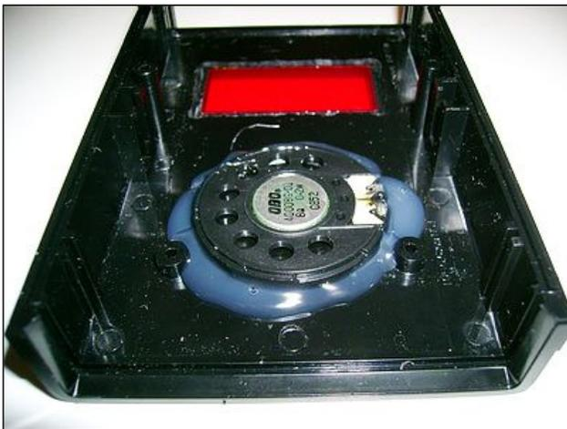
Carefully remove the two sticks, without breaking the speaker loose, and use additional hot melt glue to completely circle the edge of the speaker so that it is sealed to the front panel.
