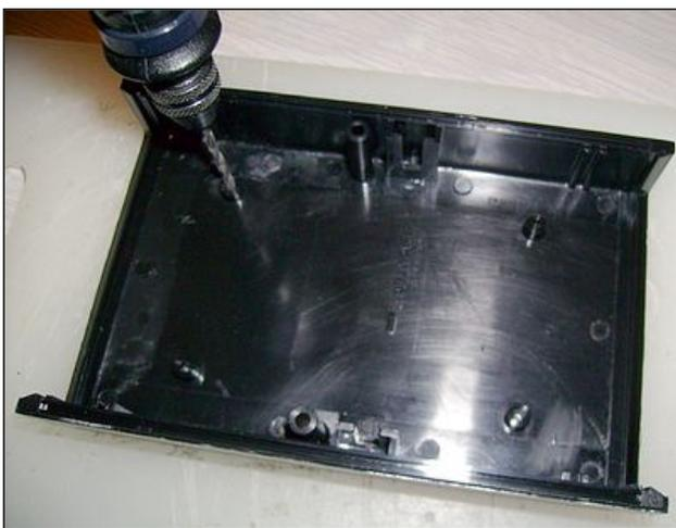
The circuit board for the Bat Scanner was designed with the Pac Tec [CM3-150](#) case in mind, though other cases could be used.
