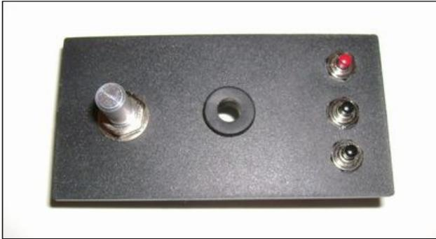
First off, I usually prepare the top panel. The function push buttons, volume control / power switch / knob and grommet for the electret microphone are generally positioned as shown. The red button is the [mode](#) button. The two black buttons are the [up](#) and [down](#) buttons.
